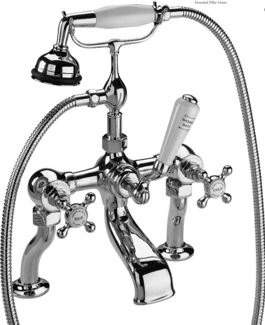
4300 Bath/spray mixer for bath rim mounting. Incorporates single check valve to comply with Water Byelaws.
